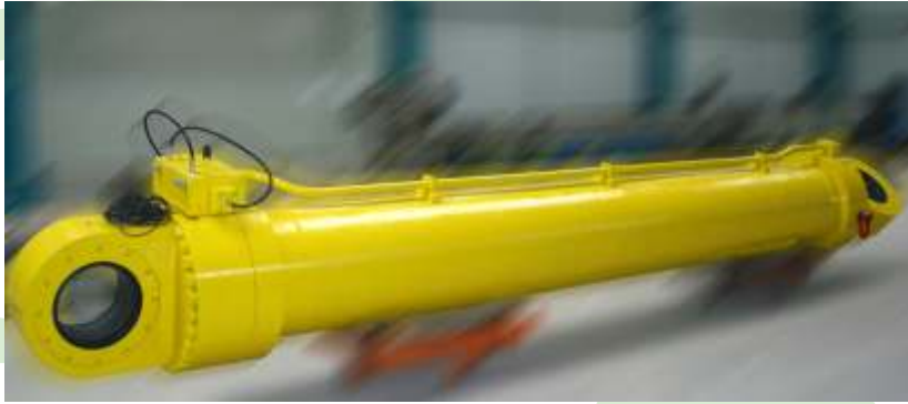
Two A-frame crane cylinders, diameter 500 mm x 350 mm, stroke 4,500 mm, fitted with hydraulic manifold and linear stroke measurement.
