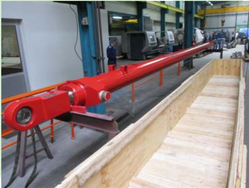
Cylinders 250 x 200 stroke 7,500 mm for telescopic boom on offshore cranes (Platforms in Africa).
