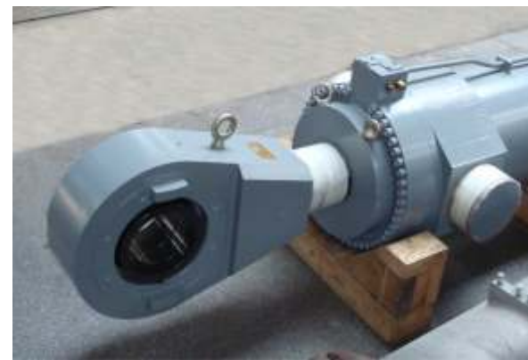
Two skidding cylinders diameter 520 mm x 250 mm, stroke 1,250 mm with ceramic coating, fitted with linear stroke measurement.
