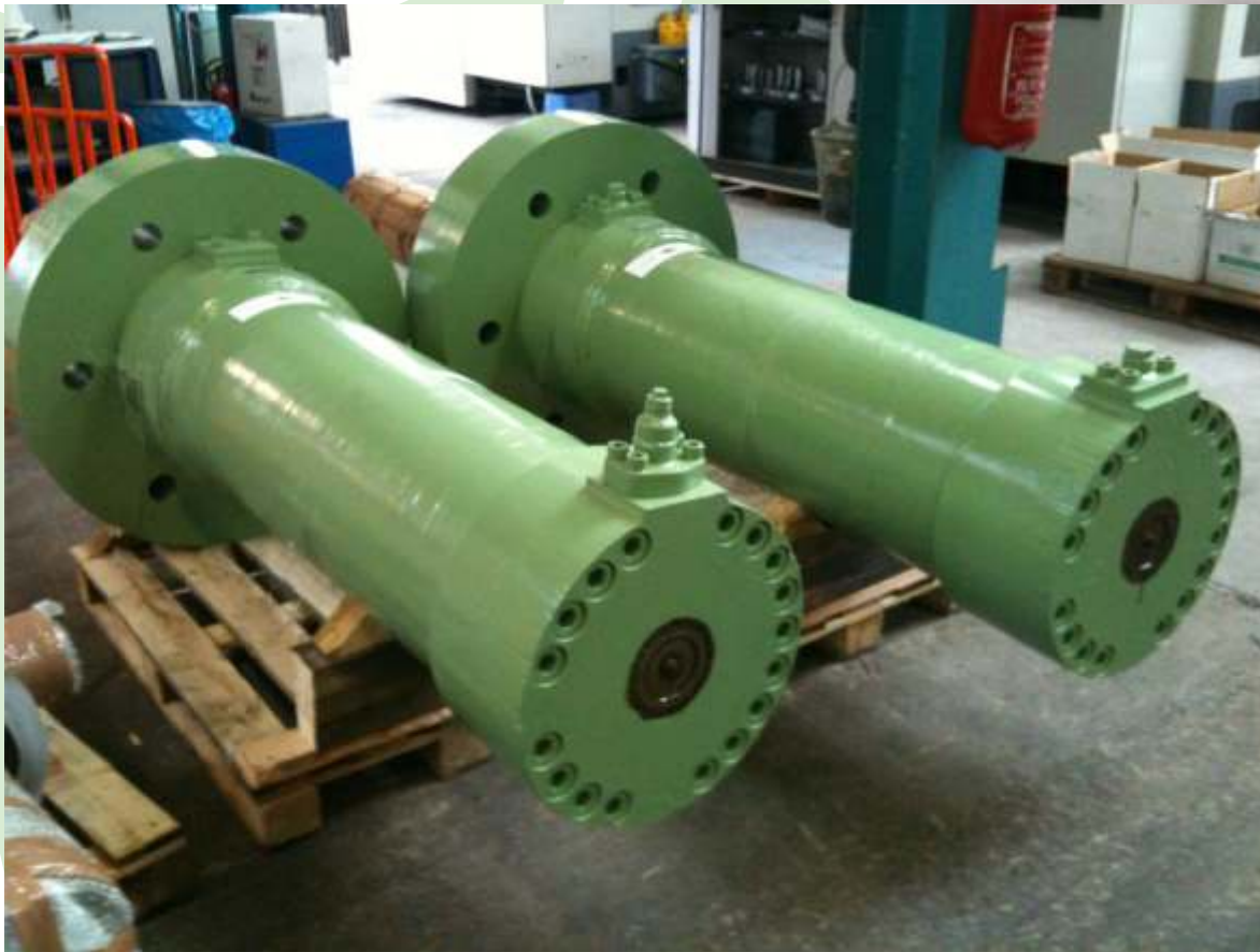
2 hydraulic cylinders diameter 360 mm x 220 mm, stroke 1,050 mm, for descaler.
