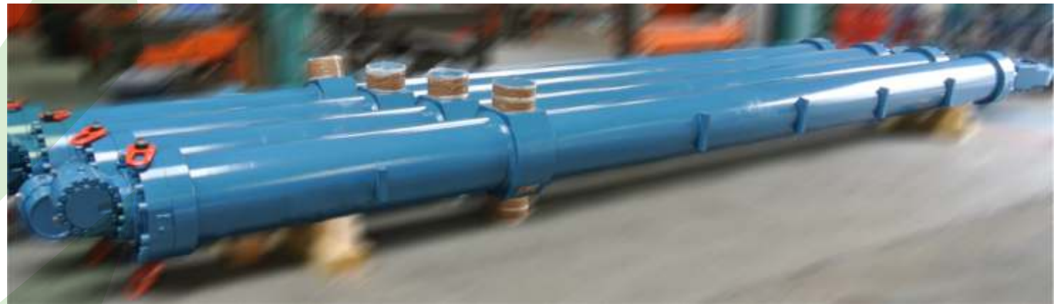
Four hydraulic cylinders, diameter 360 mm x 140 mm, stroke 7,000 mm with ceramic coating, fitted with linear stroke measurement SENSO'R.
