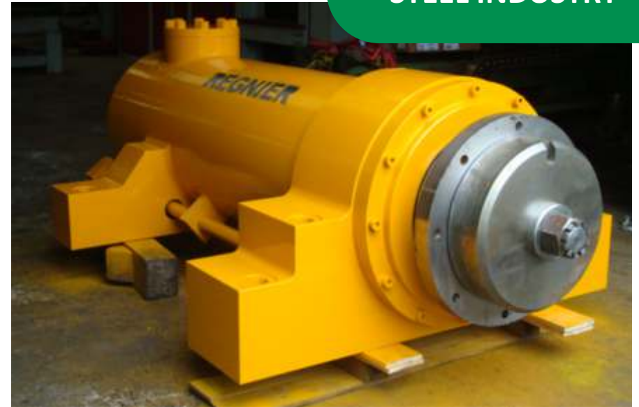
1,000 Ton hydraulic press cylinder diameter 600 mm x 560 mm, stroke 1,200 mm, with double speed design, used on straightening machines.
