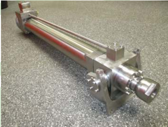
Nuclear - Hatch opening cylinder for airlocks used in the process of uranium and plutonium separation.
