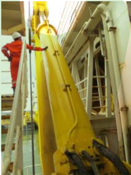
Two A-frame crane cylinders, diameter 500 mm x 350 mm, stroke 4,500 mm, fitted with hydraulic manifold and linear stroke measurement.
