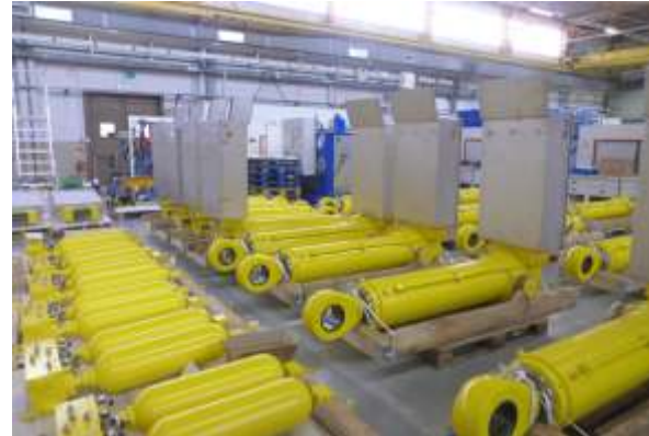
98 hydraulic cylinders, diameter 280 mm x 180 mm, stroke 1,050 mm with ceramic coating, fitted with manifolds, hydraulic controls and accumulators.
