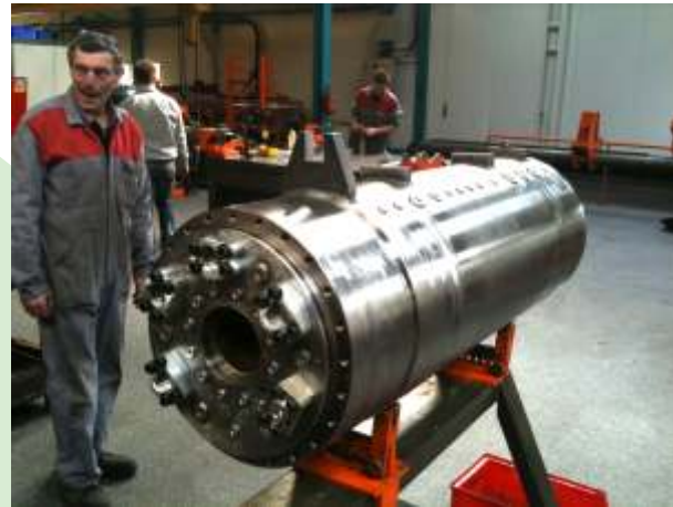
Swivel joint diameter 400 mm, 22 connections, for tunnel borer.
