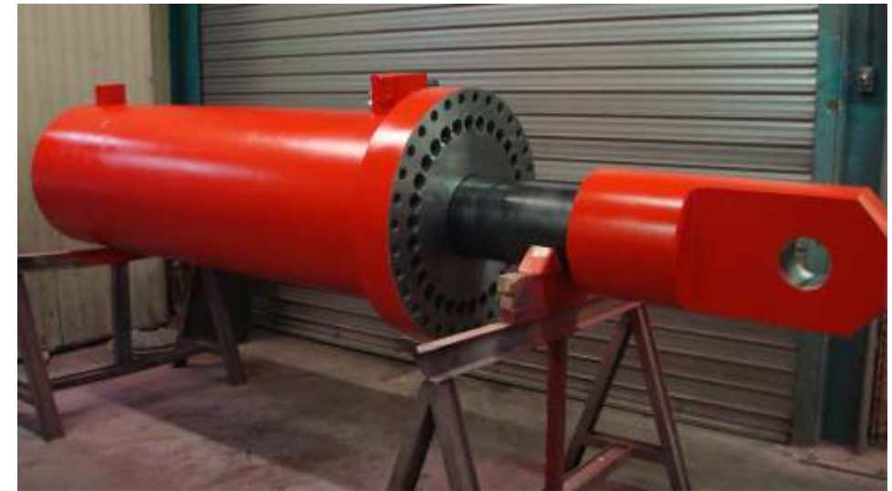
Research - Hydraulic cylinder diameter 580 mm x 280 mm, stroke 1,500 mm, for flexpipe test bench
