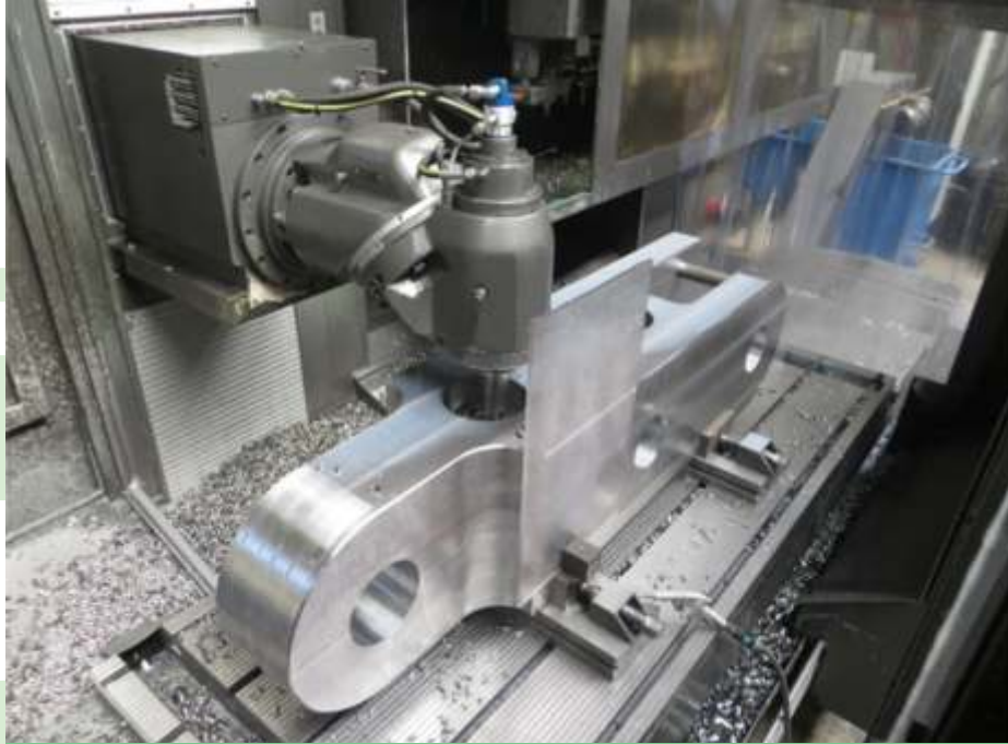
Manufacturing of forged and machine-welded frames
