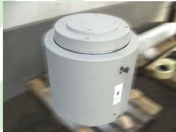
Single acting cylinder, diameter 600 mm, for crusher.
