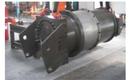
Turret lifting cylinder, diameter 655 mm x 605 mm, stroke 720 mm.
